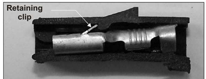
**Photo 4:** To release the terminal, depress the retaining clip and pull the terminal out from the wire end.
