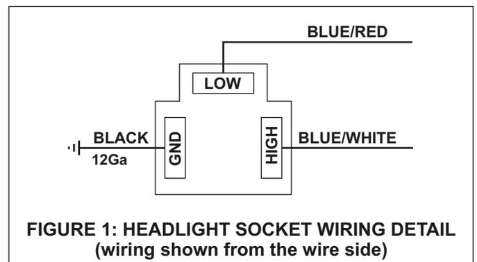
**FIGURE 1: HEADLIGHT SOCKET WIRING DETAIL (wiring shown from the wire side)**
