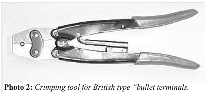
**Photo 2:** Crimping tool for British type "bullet terminals".
