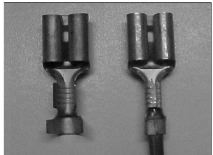
**Photo 3:** Crimp the wiring/terminals using a pair of pliers. The lower crimp should be over the insulation and the upper crimp over the bare wires only.
