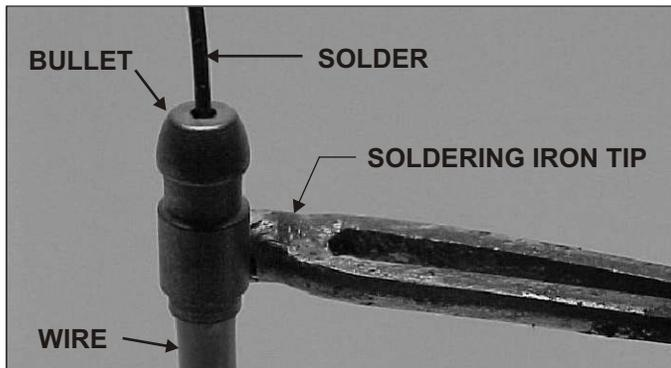
**Photo 1:** Proper technique for soldering bullet connectors
